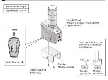
After passing the tightening screw through the bracket, attach the metal fitting.
